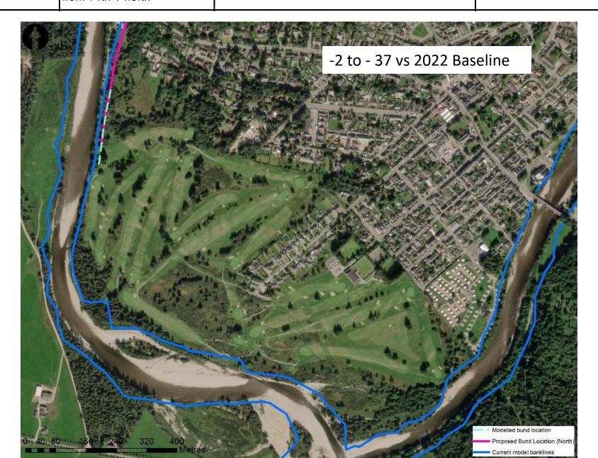
**RECOMMENDED OPTION 7** Deepening of a 330m reach of the Golf Course outlet channel by 0.5m was simulated in conjunction with a 440m long, 1.5m high bund on the left bank.
